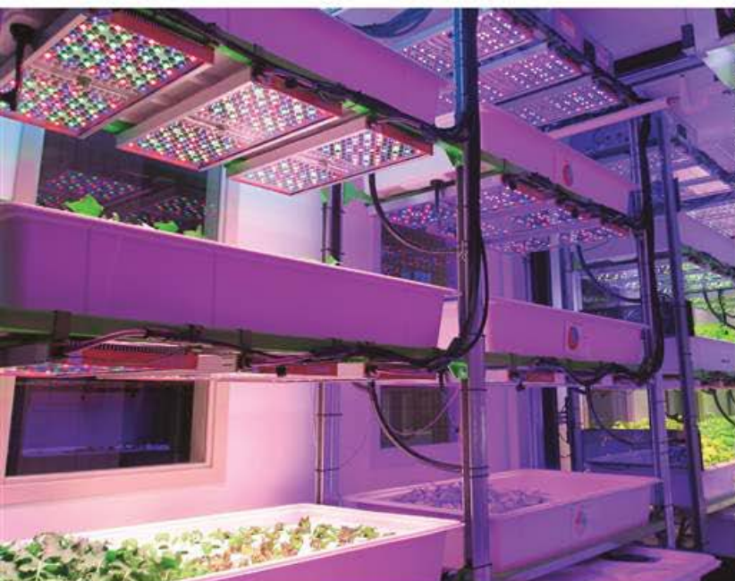
Figure 1. The Controlled-Environment Lighting Laboratory (CELL) at Michigan State University. The growth room consists of hydroponic growing racks with customizable light-emitting diodes (LEDs).
